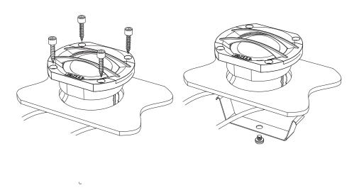
The tweeter can be mounted to a surface via the mounting cup. Choose the angle and position you prefer. Drill holes for cables and screws. After this fasten the cup with two screws. Be safe with the cables, they must be free when the tweeter is inserted into the cup.
