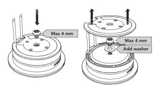
Other mounting system can be with multi holes bracket. Insert tweeter from upper side and the fixing ring from back then push all together to block the three parts. Bracket can be screwed on car factory location by side holes. There are three couple with different lengths (77, 97 and 117 mm). Cut the excess if needed. For flush mounting cut the six "bridges" that join the central ring to the side bracket of the adapter.
