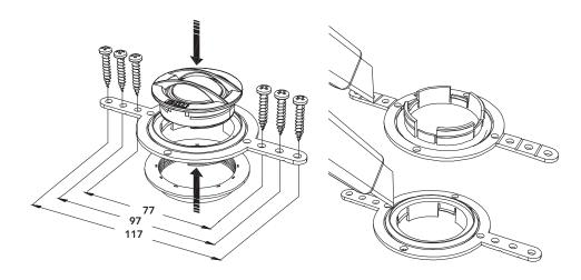
After removed the ring you can place the tweeter in a 43 mm diameter hole in a car panel (max 4 mm thickness). Place the tweeter inside the ring and push from back the fixing ring until listen the click. The outer ring can also be fixed in other ways to the car panel, for example with glue or resin, the tweeter has side hooks with which it is fixed to the ring. For similar mounting and fixing solution use the back screw to fix the metal spring.
