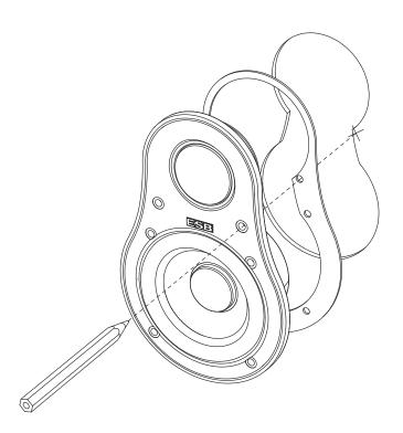
Remove the speaker and drill 2 mm holes at each mark. Connect the speaker wires, observing correct polarity, and be sure wires don't touch any metal part. Make sure the speaker is secured so that air does not leak around the mounting flange. Hand-tighten the screws evenly in a criss-cross pattern to avoid bending the speaker frame or stripping the mounting screw holes. Finally, mount the grille, insert it into the grille gap, pressing around its edge until seated firmly in the gap.
