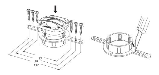
Basic mounting system is to use the four Allen screws and fix the 2.28 by the 4 mounting holes from face-plate. Similar mounting and fixing solution is to use the back screw for fix the metal spring.
