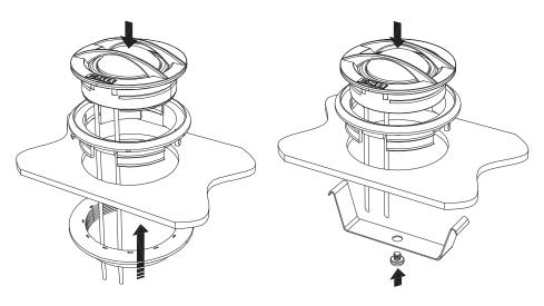
The tweeter can be mounted to a surface via the mounting cup. Choose the angle and position you prefer. Drill holes for cables and screws. After this fasten the cup with two screws. The tweeter is inserted by pressing until the click is heard. Be safe with the cables, they must be free when the tweeter is inserted into the cup.
