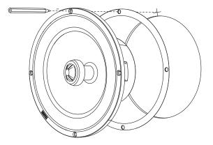
Remove the speaker and drill 2 mm holes at each mark. Connect the speaker wires, observing correct polarity, and be sure wires don't touch any metal part. Make sure the speaker is secured so that air does not leak around the mounting flange. Hand-tighten the screws evenly in a criss-cross pattern to avoid bending the speaker frame or stripping the mounting screw holes.
