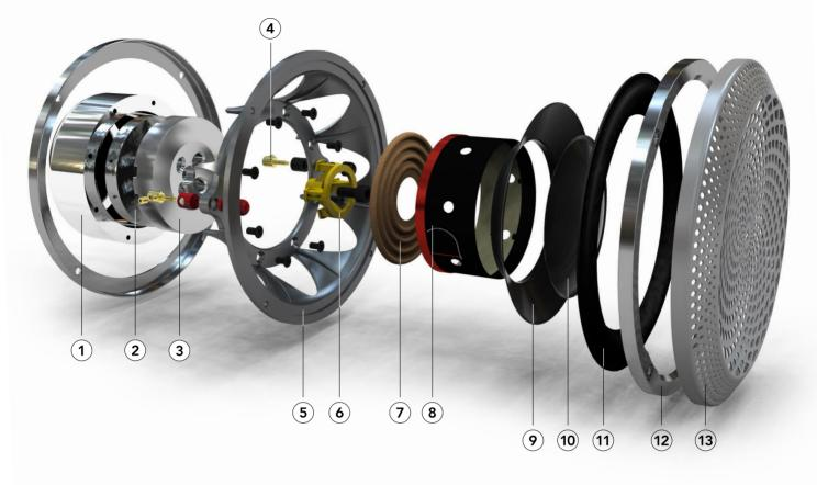
**1** Pole cup designed with the help of magnetic flux analysis software. It helped to achieve perfect and homogeneous saturation of the magnetic gap for the benefit of the voice coil stroke always immersed in constant magnetic flux, this reduces distortion and increases dynamics.
